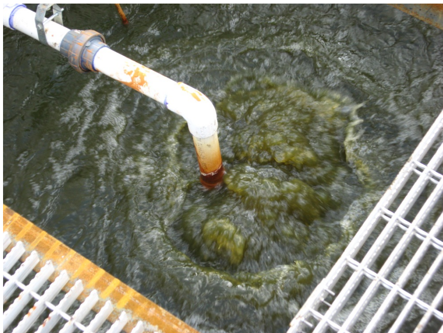
Figure 4. A-Mixer in operation.
